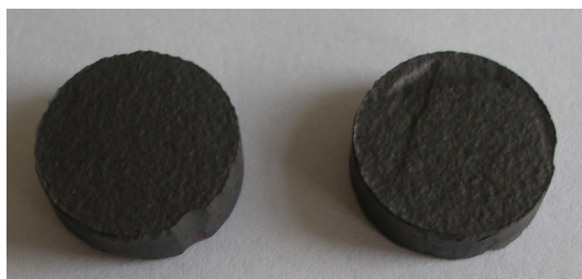
Figure 5. Double layer samples manufactured by SPS co-sintering of BSCF and NiCoCrAlY powders
